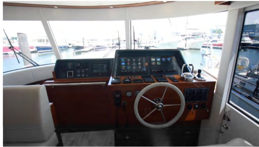
The main deck helm is starboard side mounted. The opening side door gives a full view of the side while still being able to manipulate the controls.
