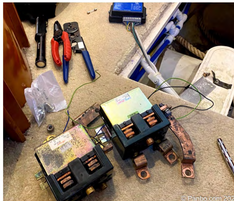
New and old solenoids side by side during the replacement of the failed one
